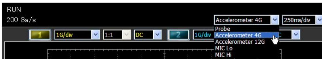
\* When using an accelerometer and removing a DC component caused by gravity, set input coupling of DEBUGSCOPE to "AC."
