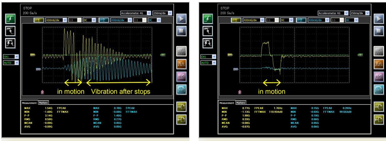
Fig. 9.2 Vibration waveform of the work
